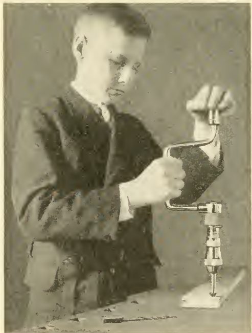
Fig. 13. Countersinking a Hole.
